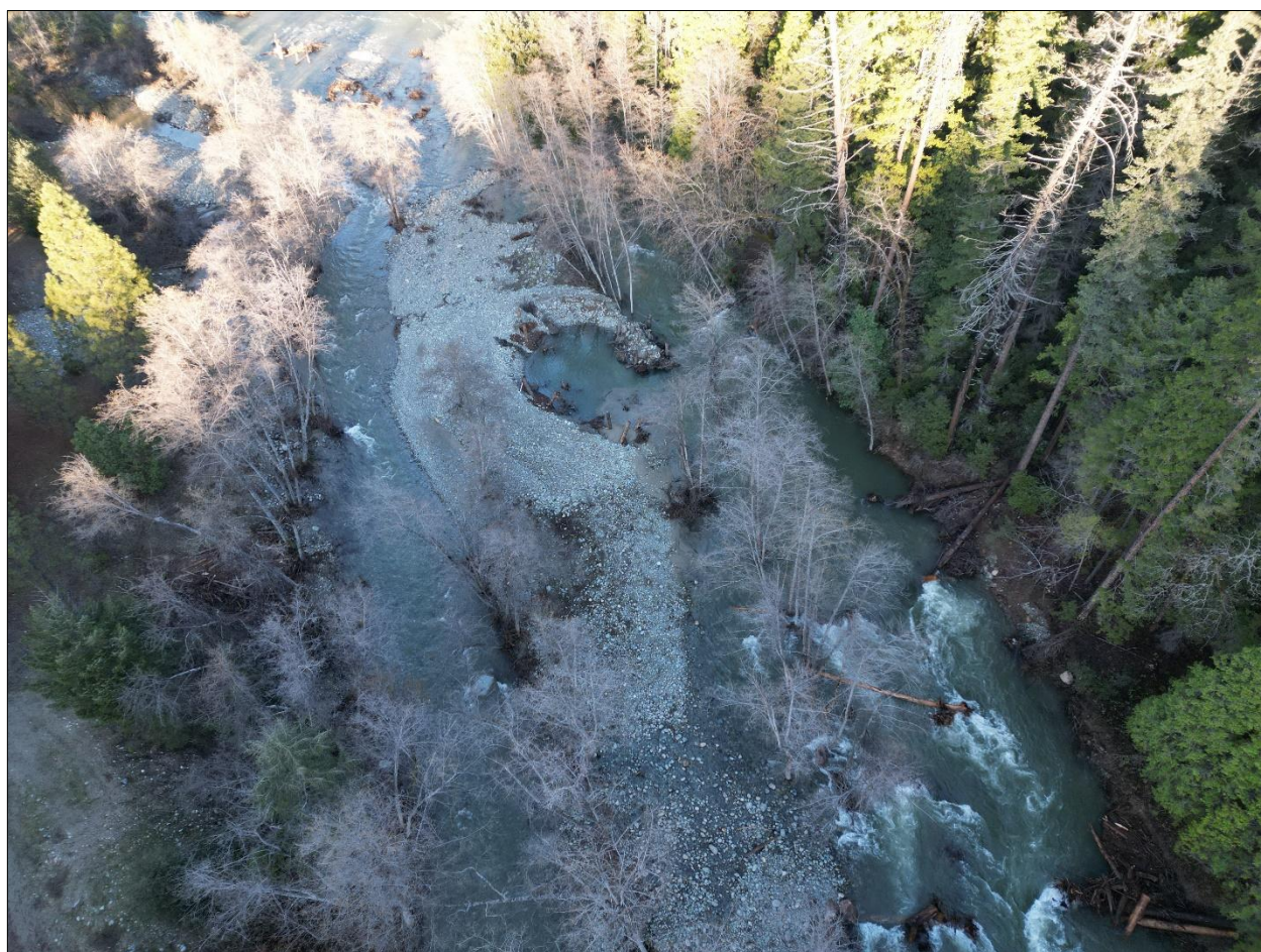
Image 10 (above): High flows on December 30 th , 2024 engaged project features and provided velocity refugia throughout the site. Note the still water in the abutment jam alcove at center. Aerial photo at approximately 16,000 CFS at the Salmon River USGS gage.
